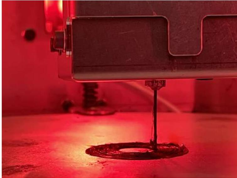
Image: Orion's Process Printing Suprem Filaprem™ CFF PEEK with TRH
