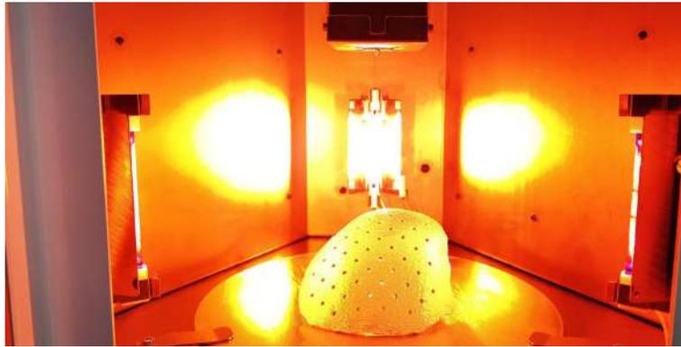
Image: Orion's Additive Manufacturing System for PEEK
