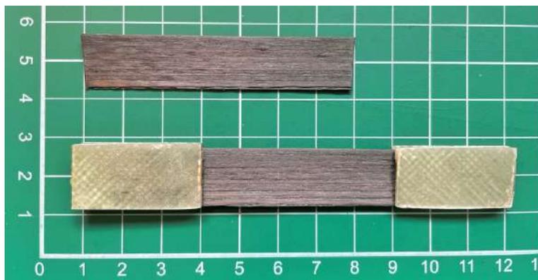
Image: Tensile Test Specimens Produced with Orion TRH Process
