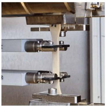
Image: Tensile Strength Tests of 3D-printed PEEK specimens printed with Orion's TRH process
