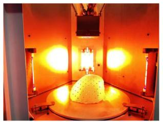
Image: PEEK Cranial Implant 3D Printed on the Orion System
